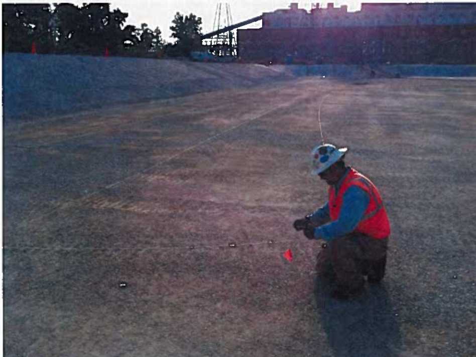
LLSI laying out a 10 foot grid on the pond floor to help keep track of data collection locations (looking northeast).
